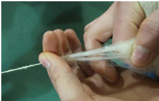
The "handler" pinches the wool with one hand and gently pulls towards her with the other to stretch the wool into just a few strands.
